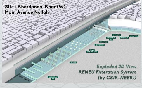
RENEU Filteration System runs across Nullah with only Anoxic Tretment covered and ECO STPs placed at existing Illegal Sewage Lines connected to Nullah.
