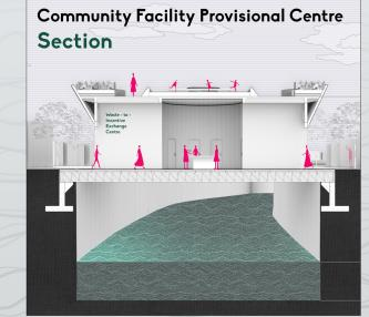
The Structure sits on a Transfer Girder, so no part of the Structure affects the flow of Nullah. Also **MODULAR** for all types of widths.
